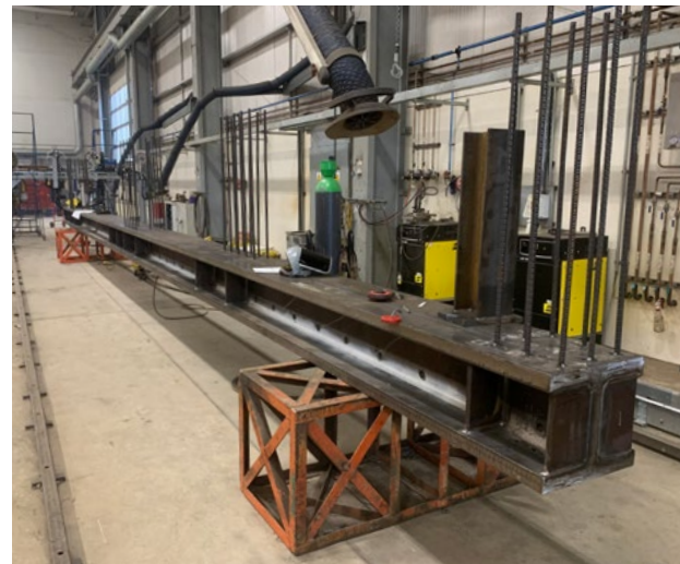
Bespoke beam fabrication, made from S460 Material - Cementation Skanska
